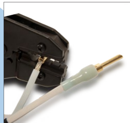
All factory crimping is performed using dedicated machine tools. The picture illustrates the process using a hand crimping tool.
